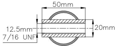
c) Each anchorage point must be able to withstand a load of 1470 daN, or 720 daN for the crotch straps.
